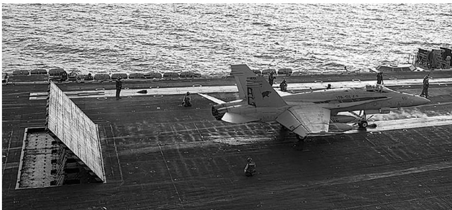
▲ JET-BLAST DEFLECTOR The deflector shield that sits behind this McDonnell Douglas F/A-18 Hornet prevents the plane's exhaust from causing damage or injury during take-off. These shields have to be strong enough to withstand temperatures close to 2,300 degrees Fahrenheit, although they are cooled by water from the sea.
